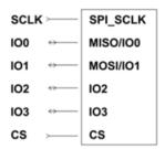
**SPI Interface** – the SPI slave interface operates up to 30MHz.
