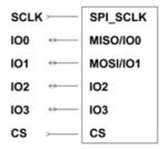
Only SPI mode 0 is supported. The SPI interface is selected by default (MODE pin is internally pulled low by 47k resistor).
