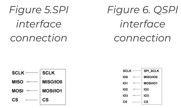
**SPI Interface** – the SPI slave interface operates up to 30MHz.
