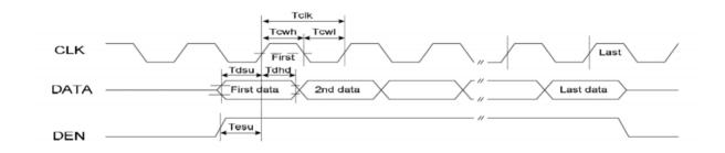
Figure 11. SYNC mode timing diagram
