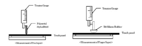
**Note 2: Measurement surface area conditions,** Scratch 100,000 times straight line on the film with a stylus change every 20,000 times with Force: 250gf, Speed: 60mm/sec by R0.8 polaceteal stylus.
