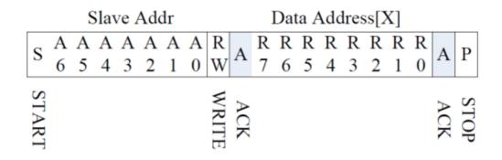
Figure 8. Read X bytes from I2C Slave
